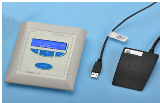
Fig. 2: electronic unit, usb cable and foot pedal, all included in the Electronic Von Frey standard package (PN 38450)
