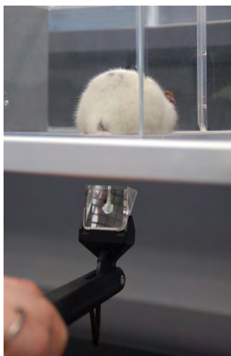
Fig. 1: "touch stimulator" transducer, including prism and protective "umbrella". Grid mesh not included (optional, PN 37450-278)
